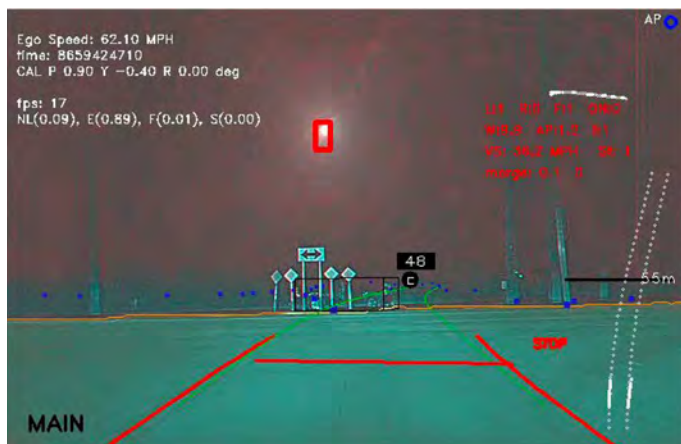
Exhibit from trial showing video feed from Tesla Model-S with overlay data showing stop line, red flashing stop line, and vehicle’s recognition of both the Tahoe and a person at or near the rear of the Tahoe. Note that the vehicle also was going 62.10 mph.
